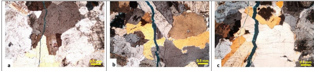
Figure 41: Microscopic view of tensile fracture under cross-polarized light: STS test with (a) displacement rate 1.5 \cdot 10^{-4} mm.s -1 , (b) displacement rate 1.5 \cdot 10^{-3} mm.s -1 , (c) displacement rate 1.5 \cdot 10^{-2} mm.s -1 .
