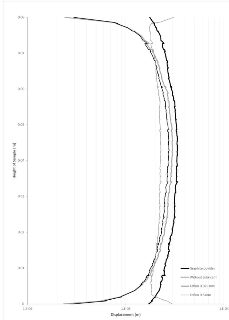
Figure 49: Specimen length vs lateral displacement of UCS test modelling without and with different lubricants.
