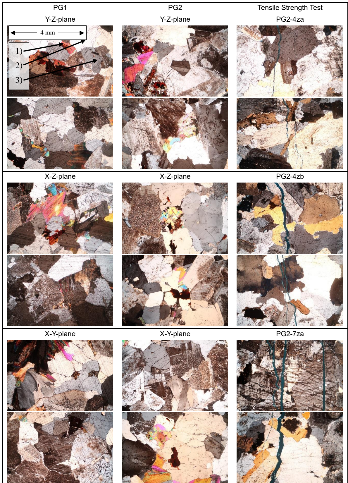
Figure 4: Optical images in cross-polarized light with 1) biotite, 2) quartz and 3) feldspar for different thin section orientations of PG1 (left), PG2 (middle) and for three different specimens tested for tensile strength after failure with loading direction from top to bottom (right). Scale is identical for all images. In thin section PG1, scratch marks are recognisable that were created during the preparation process.
